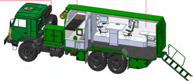
Service module 1400×2450×1520-2150 mm Living area 1330×2350×2050 mm Working area 4500×2350×2050 mm
